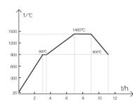
Stain & glaze sintering process (To avoid subfissure happening on bridge, the heating rate for bridge stain & glaze sintering must go down to 30°C/min)
